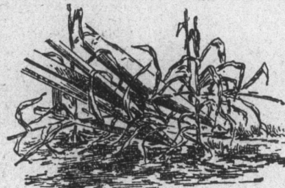
FIG. 2. TILTED FORWARD TO PICK UP LODGED CORN.
