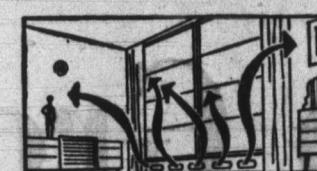
Baseboard units heat by both radiation and convection. All surfaces are warmed evenly, and control is by individual room thermostat.
