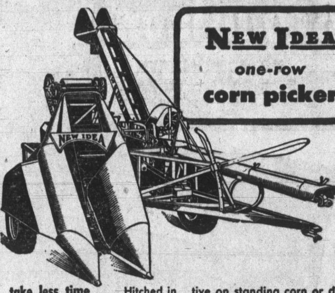
take less time . . . Hitched in a jiffy to any modern tractor. One-man operated. Picks, husks and loads up to 12 acres of corn in a day.
